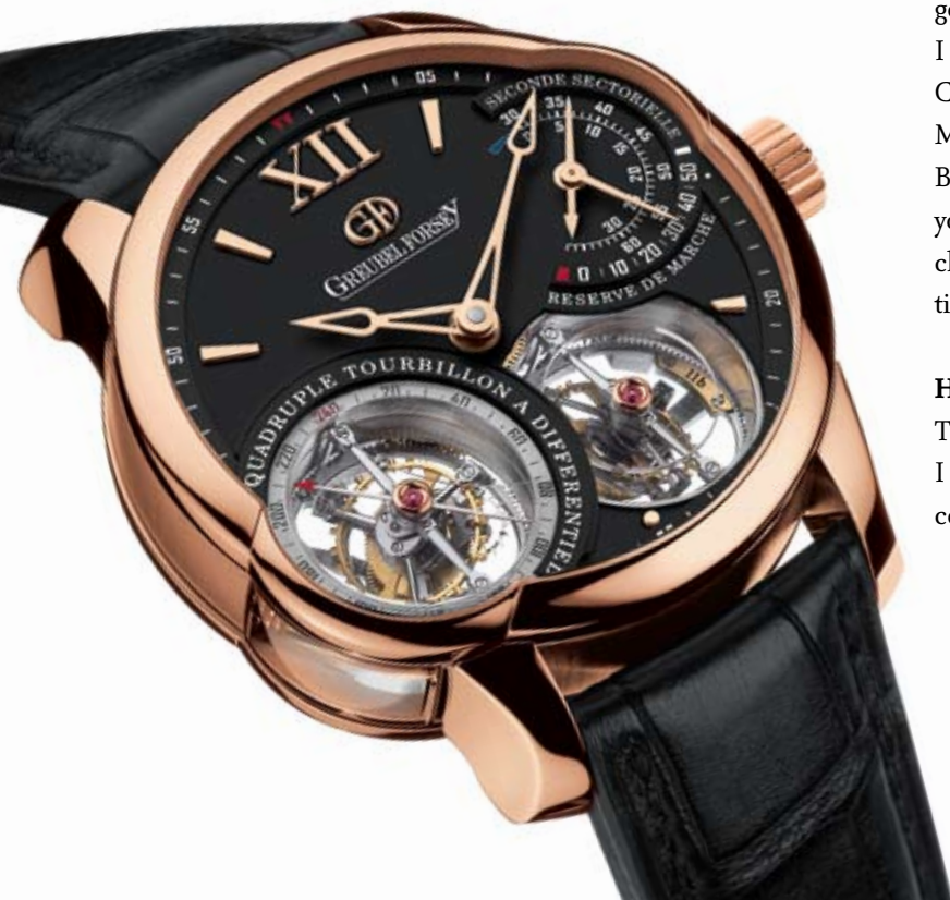
Greubel Forsey’s Quadruple Tourbillon features four fascinating asynchronous tourbillons that are linked by a spherical differential. The timepiece is available in both platinum and pink gold
